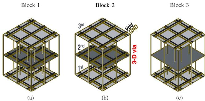
Fig. 1. Power distribution network topologies. (a) interdigitated power network on all planes with the 3-D vias distributing current on the periphery and through the middle of the circuit, (b) interdigitated power network on all planes with the 3-D vias distributing current on the periphery, and (c) interdigitated power network on planes 1 and 3 and power/ground planes on plane 2 with the 3-D vias distributing current on the periphery and through the middle of the circuit.
