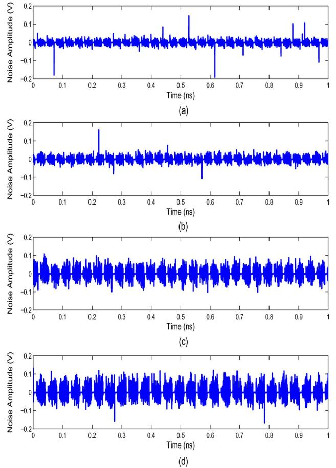
Fig. 8. Time domain measurement of the generated noise on the power line of Block 2 without board level decoupling capacitance for (a) 0 volt, (b) 0.5 volt, (c) 0.75 volt, and (d) 1 volt voltage bias on the current mirrors.
