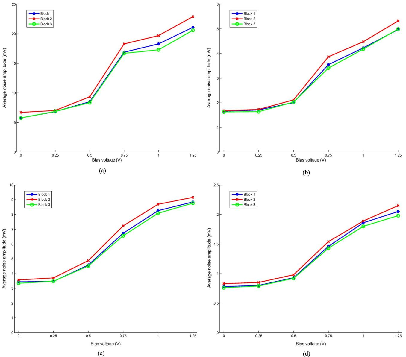
Fig. 9. Average noise voltage on the power and ground distribution networks with and without board level decoupling capacitance. (a) Average noise of power network without decoupling capacitance, (b) average noise of power network with decoupling capacitance, (c) average noise of ground network without decoupling capacitance, and (d) average noise of ground network with decoupling capacitance.
