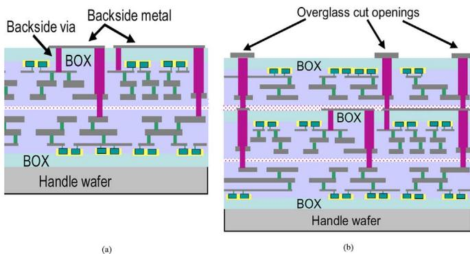
Fig. 4. Cross-sectional view of a 3-D circuit based on the MITLL process, (a) intermediate step, and (b) fully fabricated 3-D stack [14]. The second plane is flipped and bonded with the first plane, while the third plane is bonded face-to-back with the second plane. The backside metal layer, vias, and through silicon vias are also shown [14].
