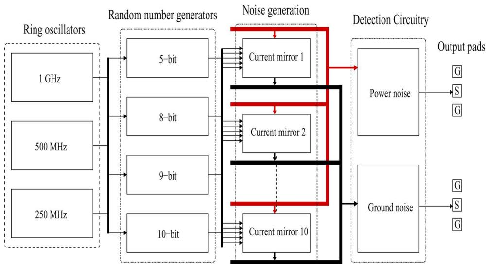
Fig. 2. Block level schematic of noise generation and detection circuits.
