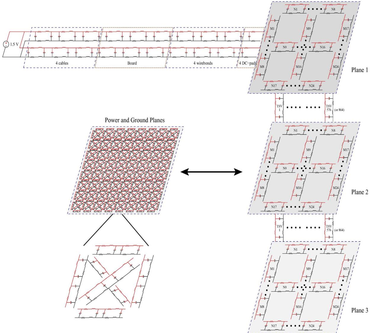
Fig. 11. Equivalent electrical model of the cables, board, wirebonds, on-chip DC pads, power distribution networks, and TSVs.
