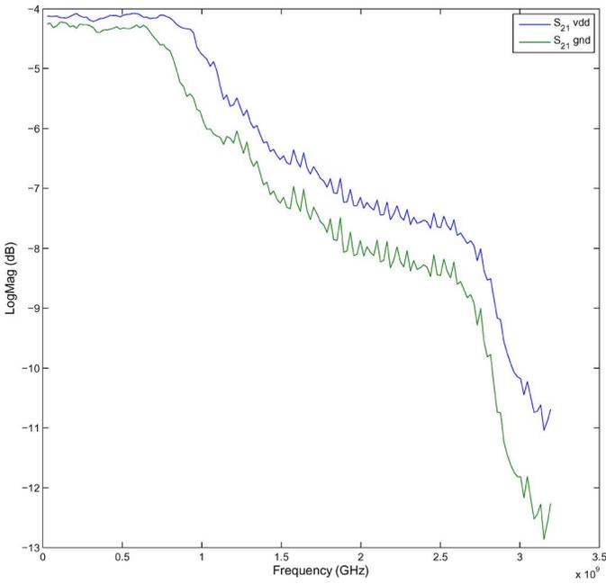
Fig. 6. S-parameter characterization of the power and ground noise detection circuits.
