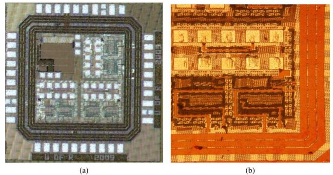
Fig. 5. Fabricated test circuit examining noise propagation for three different power distribution networks and a distributed DC-to-DC rectifier, (a) die microphotograph of the 3-D test circuit, and (b) an enlarged image of Block 1.
