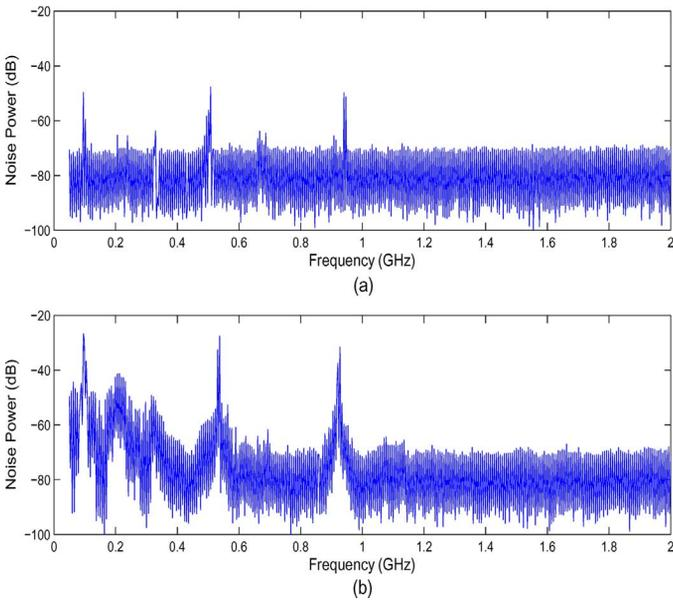
Fig. 7. Spectral analysis of the noise generated on the power line of Block 2 with (a) board level decoupling capacitance, and (b) without board level decoupling capacitance.
