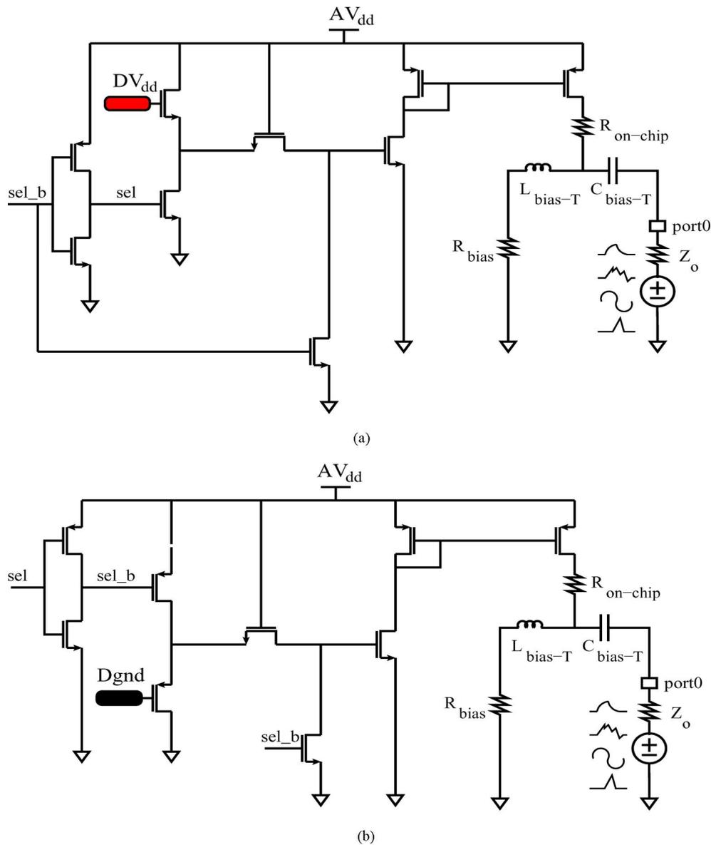
Fig. 3. Source-follower noise detection circuits that detect noise on both the digital (a) power lines, and (b) ground lines.
