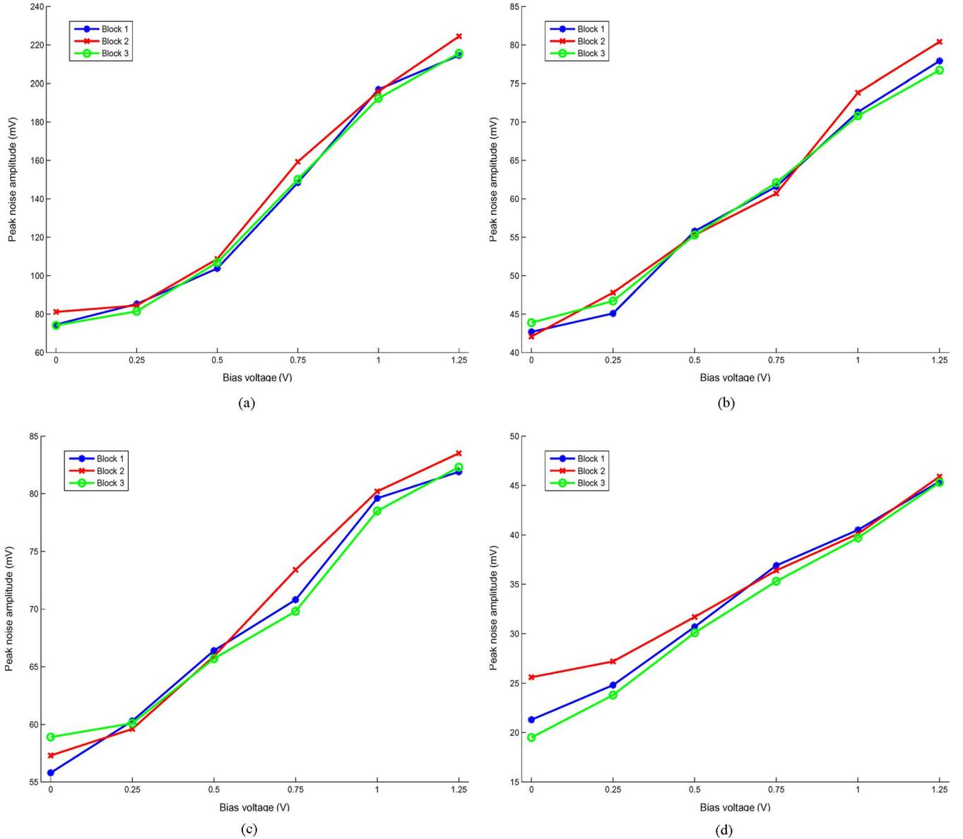
Fig. 10. Peak noise voltage on the power and ground distribution networks with and without board level decoupling capacitance. (a) Peak noise of power network without decoupling capacitance, (b) peak noise of power network with decoupling capacitance, (c) peak noise of ground network without decoupling capacitance, and (d) peak noise of ground network with decoupling capacitance.
