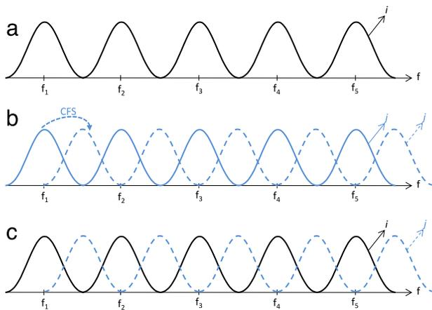
**Fig. 1.** Users  $i$  and  $j$  fully overlap by allocating the same resources at the same time in (a) and (b) (solid curves), respectively.  $j$  performs CFS to decrease the interference in (b) (dashed curve).  $i$  and  $j$  partially overlap in (c).
