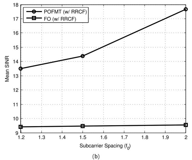
**Fig. 5.** CDF of the SINR values achieved in orthogonal waveforms with RRC filter for various the subcarrier spacing values. (a) When filter roll-off is constant, increasing the subcarrier spacing increases the SINR gain. (b) When the subcarrier spacing increases, i.e., in other words, when the bandwidth usage rises, mean SINR level also increases.
