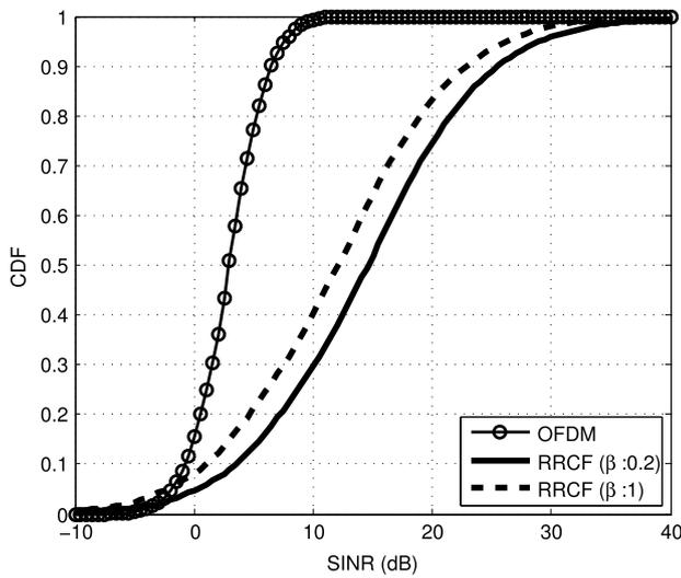
**Fig. 3.** CDF of the SINR values achieved in orthogonal waveforms with RRC filter for various the roll-off values. When subcarrier spacing is constant, increasing the filter roll-off decreases the SINR gain.
