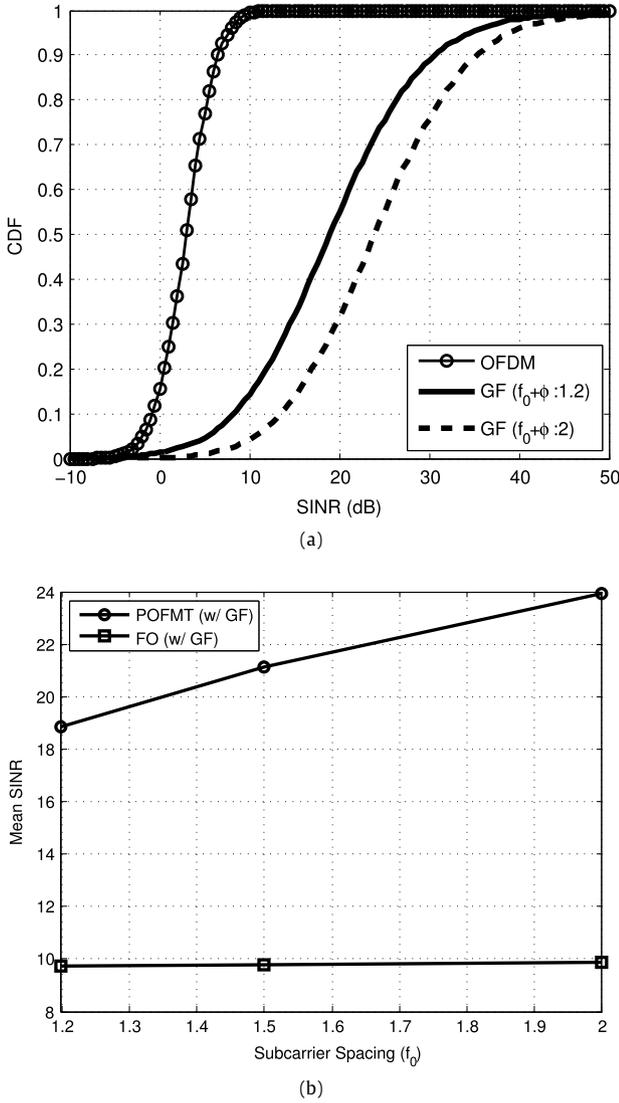
**Fig. 6.** CDF of the SINR values achieved in non-orthogonal waveforms with Gaussian filter for various the subcarrier spacing values. (a) When filter control parameter is constant, increasing the subcarrier spacing increases the SINR gain. (b) When the subcarrier spacing increases, i.e., in other words, when the bandwidth usage rises, mean SINR level also increases.
