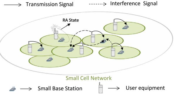
**Fig. 2.** System view. In uncoordinated network structure, the system has multiple small BSs with a single user. Also, each user has RA which can form a state in one direction.
