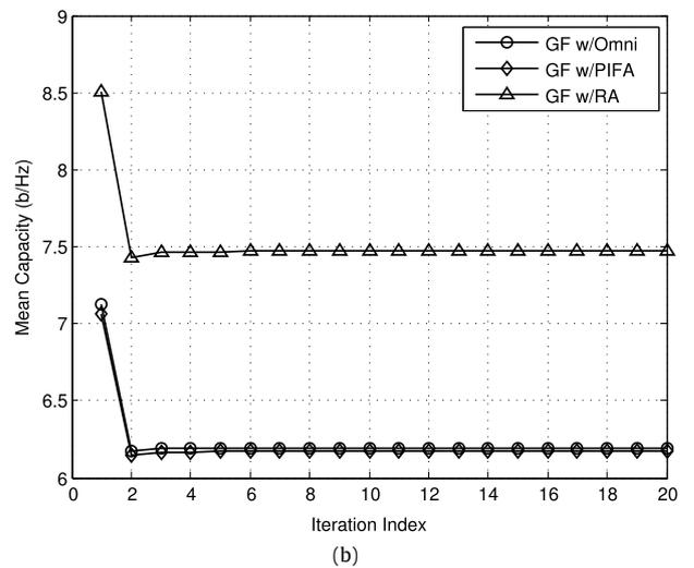
**Fig. 7.** Mean capacity values in each iteration for orthogonal waveforms with RRC filter. (a) When RAs are used within POT concept, the system gain can be increased further in orthogonal schemes. (b) The system with orthogonal scheme and RA can reach the NE.
