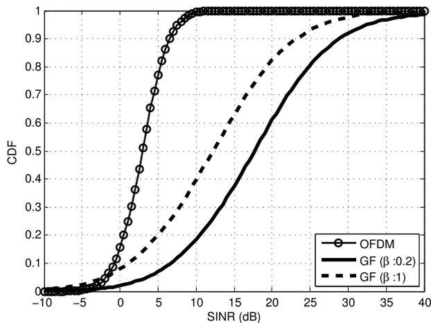
**Fig. 4.** CDF of the SINR values achieved in non-orthogonal waveforms with Gaussian filter for various the roll-off values. When subcarrier spacing is constant, increasing the filter control parameter decreases the SINR gain in non-orthogonal waveforms with Gaussian filter.
