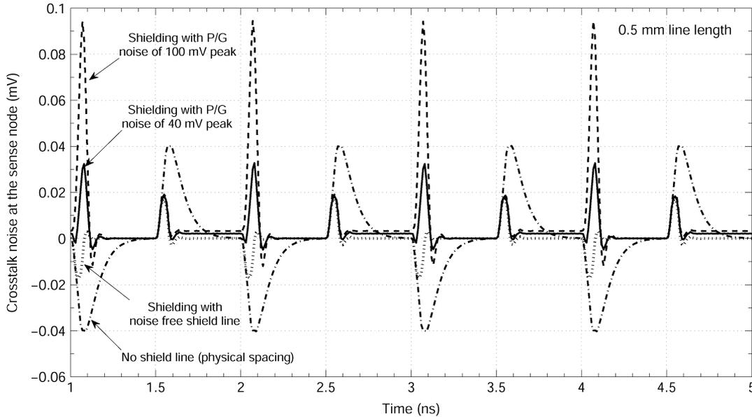
Fig. 15. Crosstalk noise at the sense node with an inserted shield line with different noise profiles (noise free, 40, and 100 mV P/G noise on the shield line) and without a shield line (physical spacing). The interconnect length is 0.5 mm.
