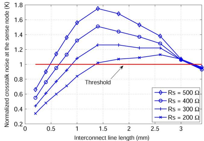
Fig. 7. Effect of interconnect length on crosstalk noise at the sense node for several driver sizes.
