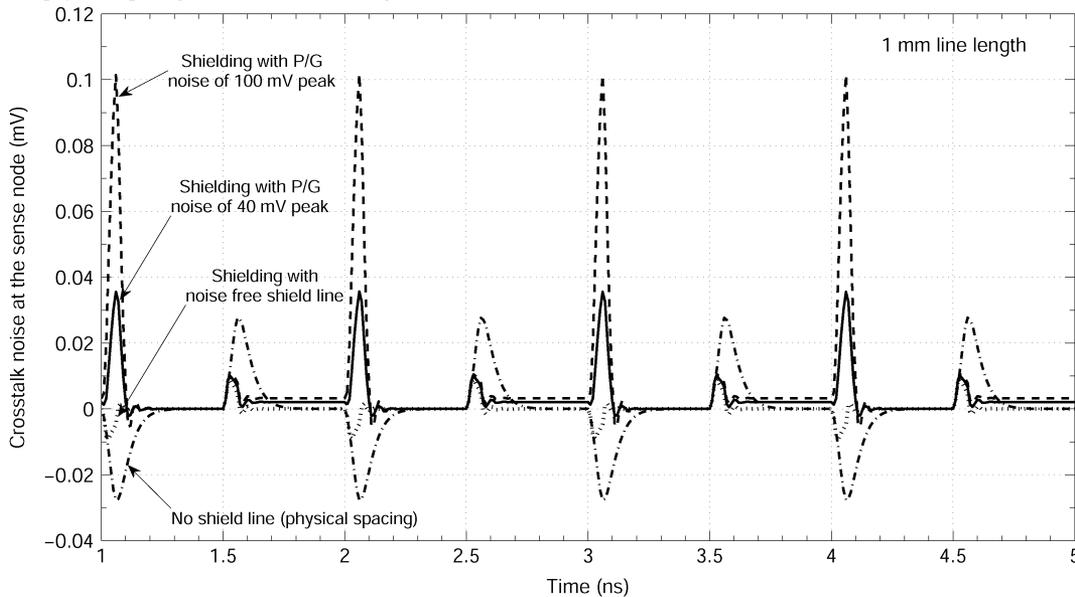
Fig. 16. Crosstalk noise at the sense node with an inserted shield line with different noise profiles (noise free, 40, and 100 mV P/G noise on the shield line) and without a shield line (physical spacing). The interconnect length is 1 mm.
