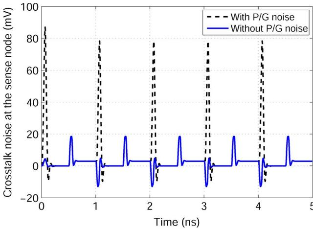
Fig. 4. Crosstalk noise at the sense node with a noisy shield line and a noise free shield line. Note that the crosstalk noise increases dramatically when P/G noise is present on the shield line.
