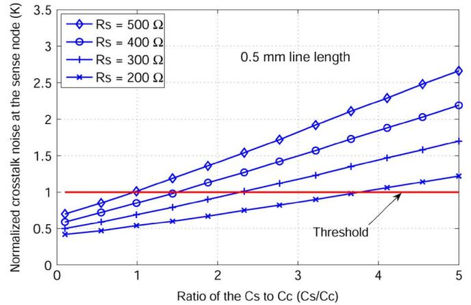
Fig. 11. Ratio of substrate capacitance to coupling capacitance versus normalized crosstalk noise when a P/G line is routed as a shield line. The interconnect length is 0.5 mm.
