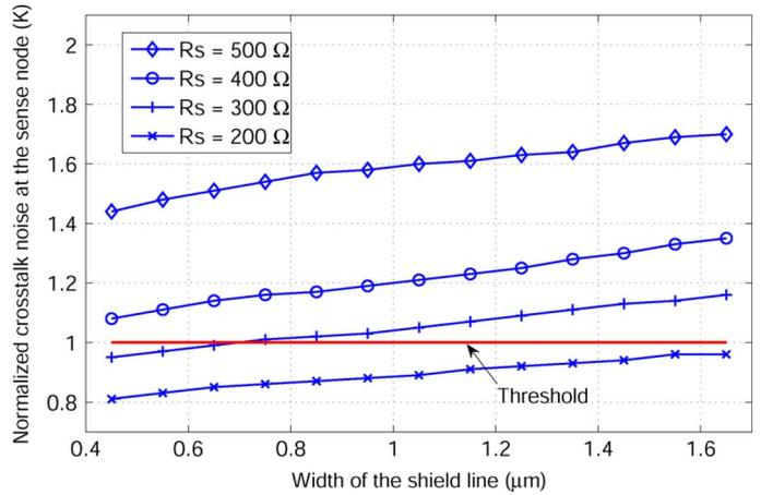
Fig. 9. Effect of shield line width on crosstalk noise for a 1 mm interconnect line. Note that signal integrity with shield insertion is degraded above the threshold line.
