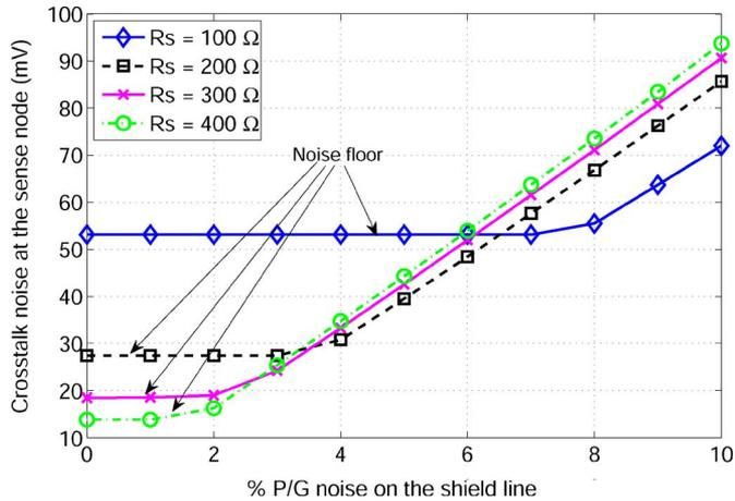
Fig. 5. Crosstalk noise at the sense node as the P/G noise is varied from 0% to 10% of the supply voltage for different driver resistances. Note that a noise floor exist for each driver resistance. This noise floor is due to the noise coupled from the aggressor line to the victim line when P/G noise is less than 7% of the supply voltage with a small driver (i.e., driver resistance is 400  $\Omega$ ) and less than 2% with a large driver (i.e., driver resistance is 100  $\Omega$ ).
