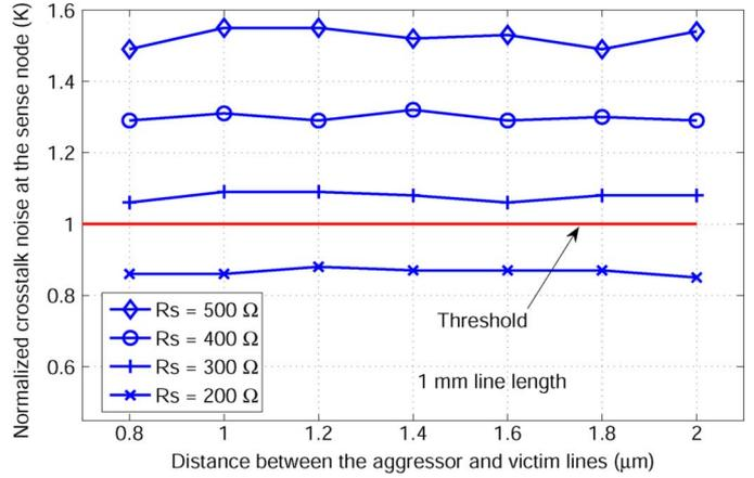
Fig. 14. Normalized crosstalk noise when a P/G line is routed as a shield line where the distance between the aggressor and victim line is varied from 0.8 to 2  $\mu\text{m}$ . The interconnect length is 1 mm.
