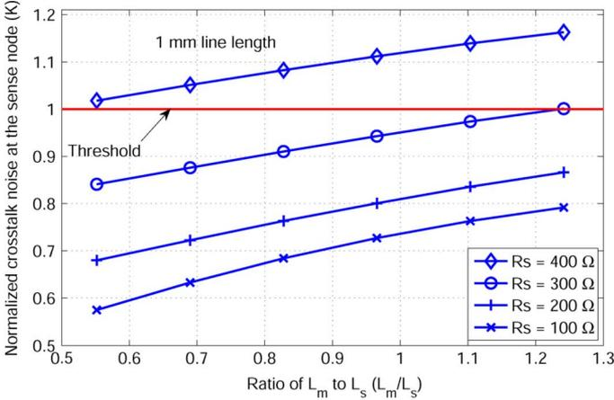
Fig. 13. Ratio of self-inductance to mutual inductance versus normalized crosstalk noise when a P/G line is routed as a shield line. The interconnect length is 1 mm.
