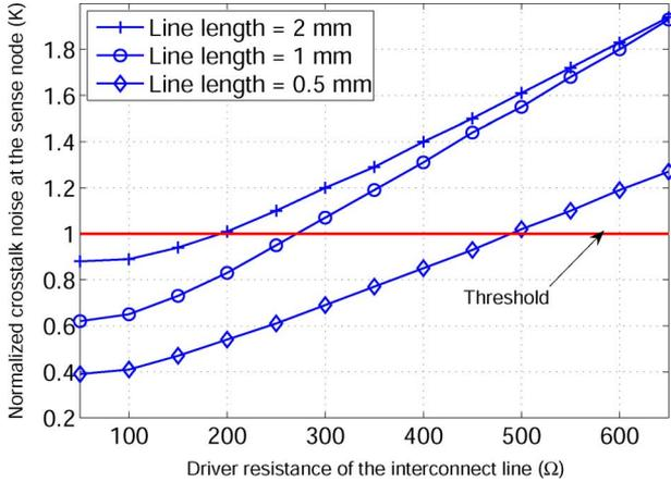
Fig. 10. Effect of  $R_{line}/R_s$  on the crosstalk noise voltage. The length of the interconnect line is 0.5, 1, and 2 mm.
