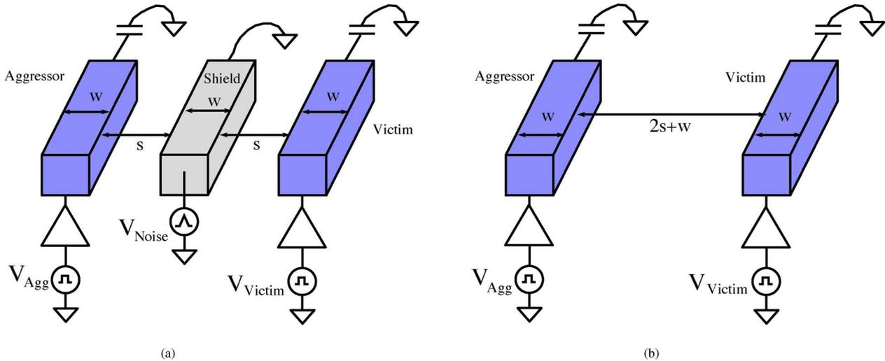
Fig. 1. Global interconnect model for (a) shield line between an aggressor and victim line and (b) physical spacing between an aggressor and victim line. The aggressor and victim lines are modeled with a driver resistance at the near end and terminated with a load capacitance at the far end. P/G noise is modeled as a single voltage source at the near end of the shield line.
