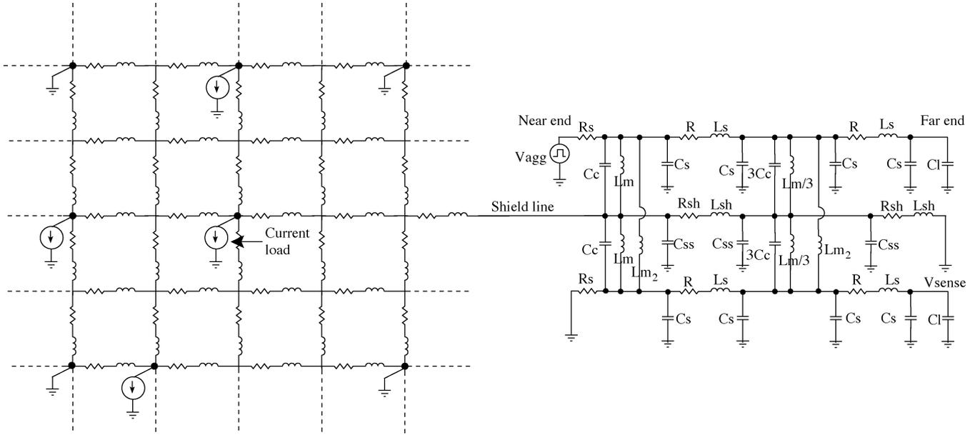
Fig. 3. Ground distribution network used as shield lines to evaluate the effects of P/G noise on the crosstalk noise at the sense node for passive shielding. The ground distribution network consists of multiple ground connections and the current loads are modeled as active devices connected to the ground network.
