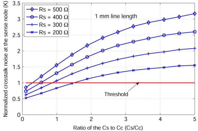
Fig. 12. Ratio of substrate capacitance to coupling capacitance versus normalized crosstalk noise when a P/G line is routed as a shield line. The interconnect length is 1 mm.
