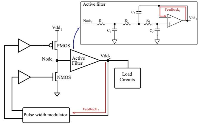
Fig. 3. Proposed DC-DC converter. Note that the passive LC filter is replaced with an active filter and the large tapered buffers are no longer necessary.
