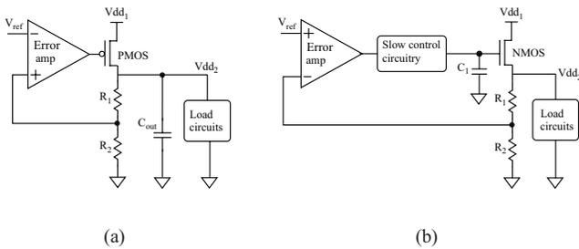
Fig. 1. LDO voltage regulators (a) with a PMOS output stage where  $R_1$  and  $R_2$  are adjusted to generate a different dc voltage at the output and (b) with an NMOS source follower output stage where  $C_1$  is connected to the gate of the NMOS transistor to reduce coupling from the output to the gate terminal.
