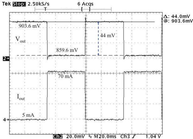
Fig. 11. Measured load regulation when the transient output current changes between 5 and 70 mA. The output dc voltage shift is 44 mV. The transition time of the output current is approximately 70 ns.
