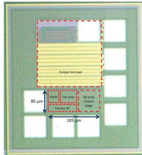
Fig. 7. Die microphotograph of the hybrid voltage regulator.
